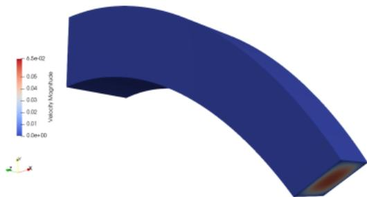
The average pressure, estimated by our program, is 7% lower than the average value on the inlet face for OpenFoam. Instead the axial velocity is 4% higher.
